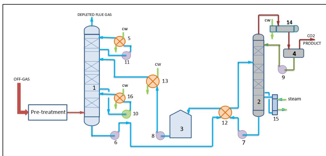
1- Absorber, 2- Stripper, 3- Lean amine tank, 4- Reflux accumulator, 5- Wash water cooler, 6- Rich amine pump, 7- Lean amine pump, 8- Absorber feed pump, 9- Reflux pump, 10- Intercooler pump, 11- Wash water pump, 12- Lean/Rich Heat exchanger, 13- Lean amine cooler, 14- Condenser, 15- Reboiler, 16- Inter cooler
